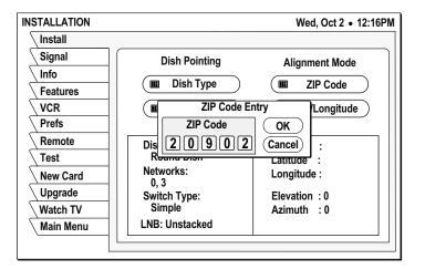
The correct azimuth and elevation angles will appear with onscreen instructions for using these values to properly align your dish antenna.
